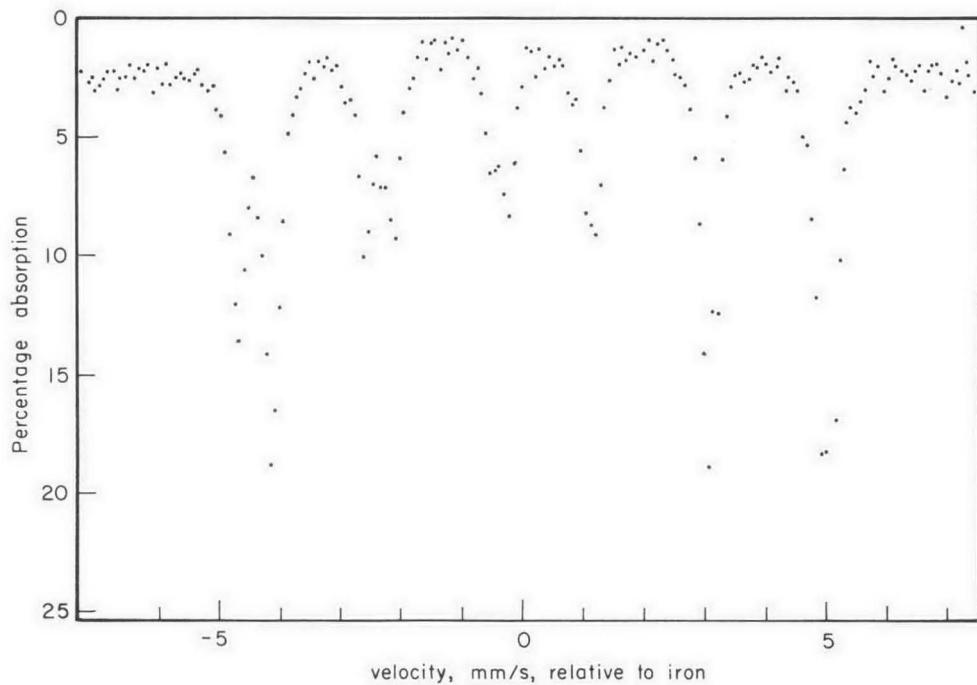
Figure 4.  $^{57}\text{Fe}$  spectrum of synthetic magnetite,  $\text{Fe}_3\text{O}_4$ , at room temperature. Note the evidence for at least two different iron sites, with different magnetic fields and isomer shifts.
